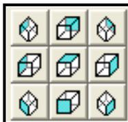
Clicking on a View button will show a view of the 3D “wire-frame” model. The view will be of the shape as seen from the colored side of the cube symbol. For example, the center button, with the colored side of the cube at the top displays a Top View of the model. The lower right button displays an Isometric view from the right-front angle.
